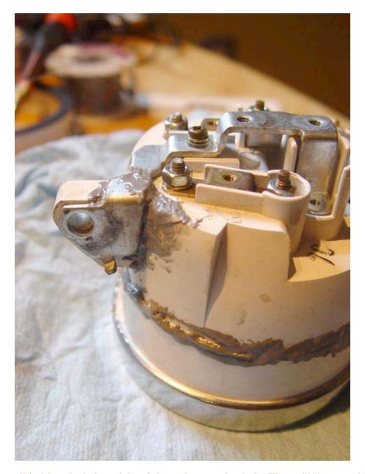
Note the small 'tab' to the below right of the tach mounting hole. That will line up with a small slot on the bike.
